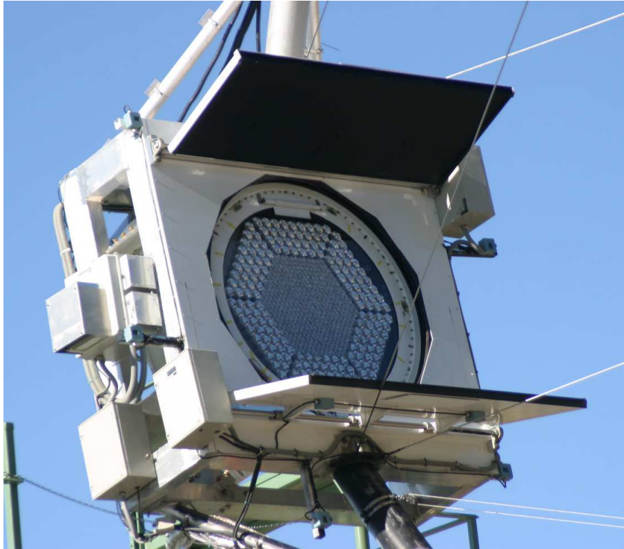
Figure 2.8: Front view of the MAGIC Telescope camera. Several parts of the camera can be observed in this photograph: the protecting plexiglass window, the light concentrators collect the incident light onto the camera photosensors as well as other most exterior elements like the camera lids.
