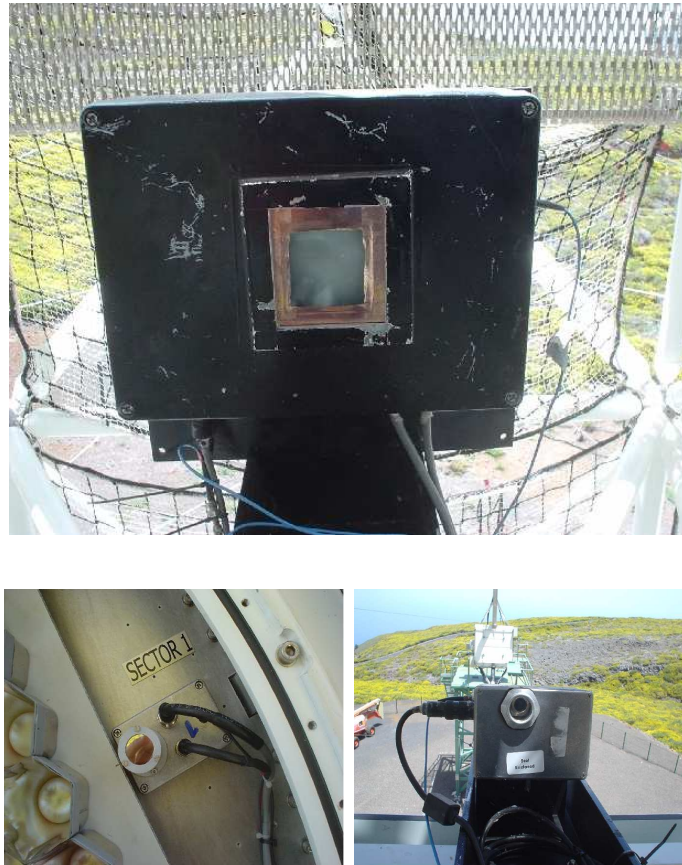
Figure 2.12: Picture of the main components of the MAGIC calibration system. The top picture shows a front view of the pulser box when installed in the central part of the reflector dish. Whereas the bottom left picture shows the on of the blind pixels installed in the camera and the the bottom right the PIN diode installed around one meter in front of the pulser box . Notice that in this last picture it is possible to see the MAGIC camera in the rear part of the picture.
