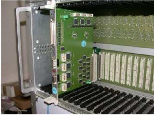
**Figure 2:** One LT1-board plugged in the Backplane.
