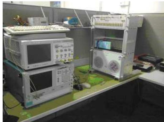
**Figure 4:** On the left of the picture the Signal Generator and the oscilloscope, while on the right the LT1 system, lacking of LT1-boards.
