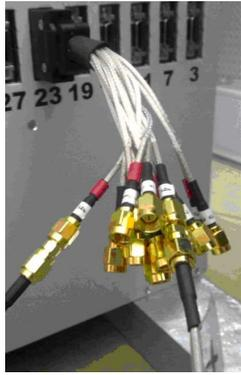
**Figure 9:** An image of the connector used to adapt SMA to MDR format.
