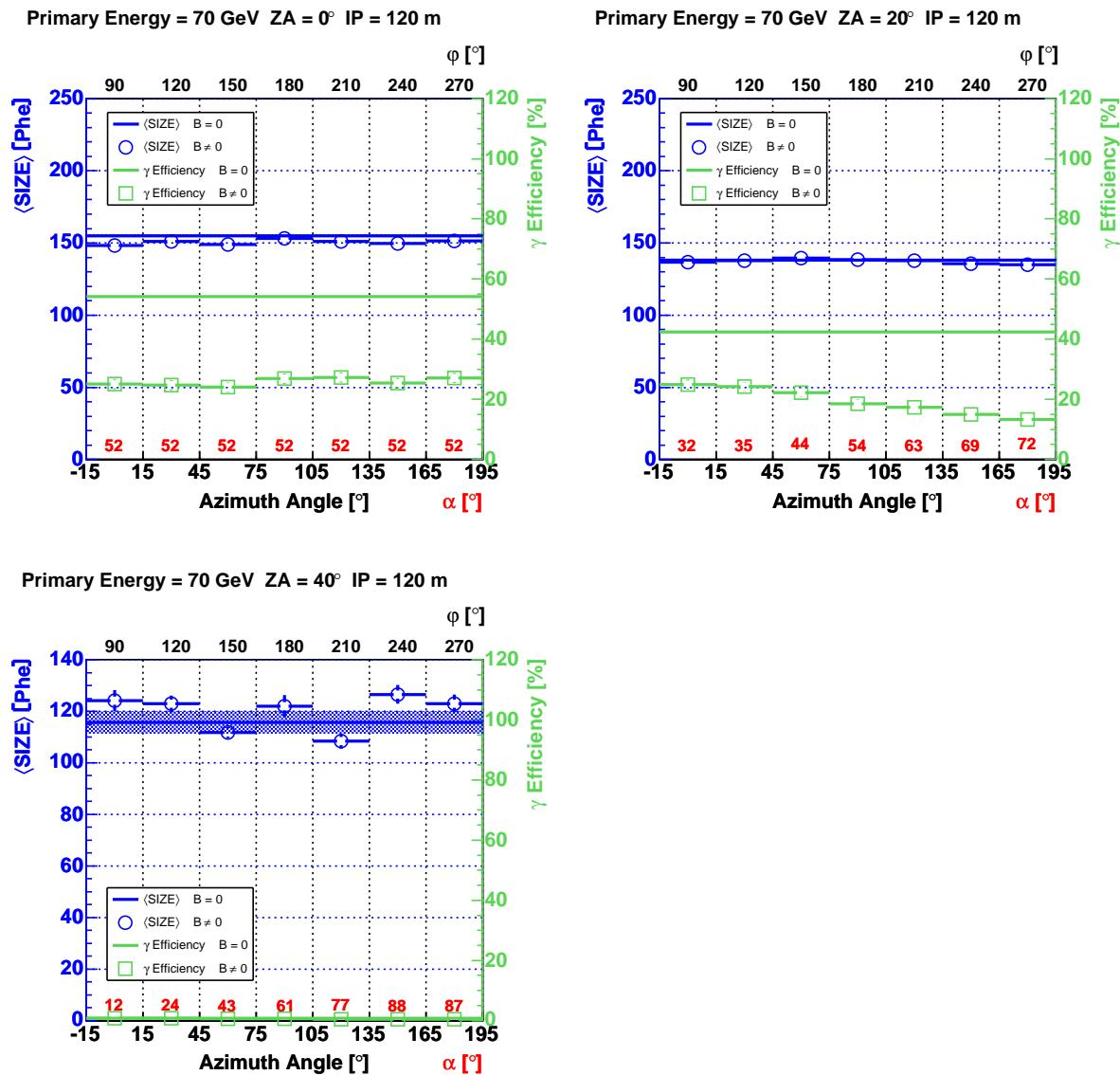
**Figure 203:** The mean value of the image parameter SIZE and the  $\gamma$  efficiency as a function of the azimuth angle for 70 GeV  $\gamma$ -rays and ZA between  $0^\circ$  and  $40^\circ$ . The telescope is always placed at angles  $\varphi = \text{azimuth angle} + 90^\circ$ . The impact parameter was set to  $r = 120$  m. The hard image cleaning was applied.
