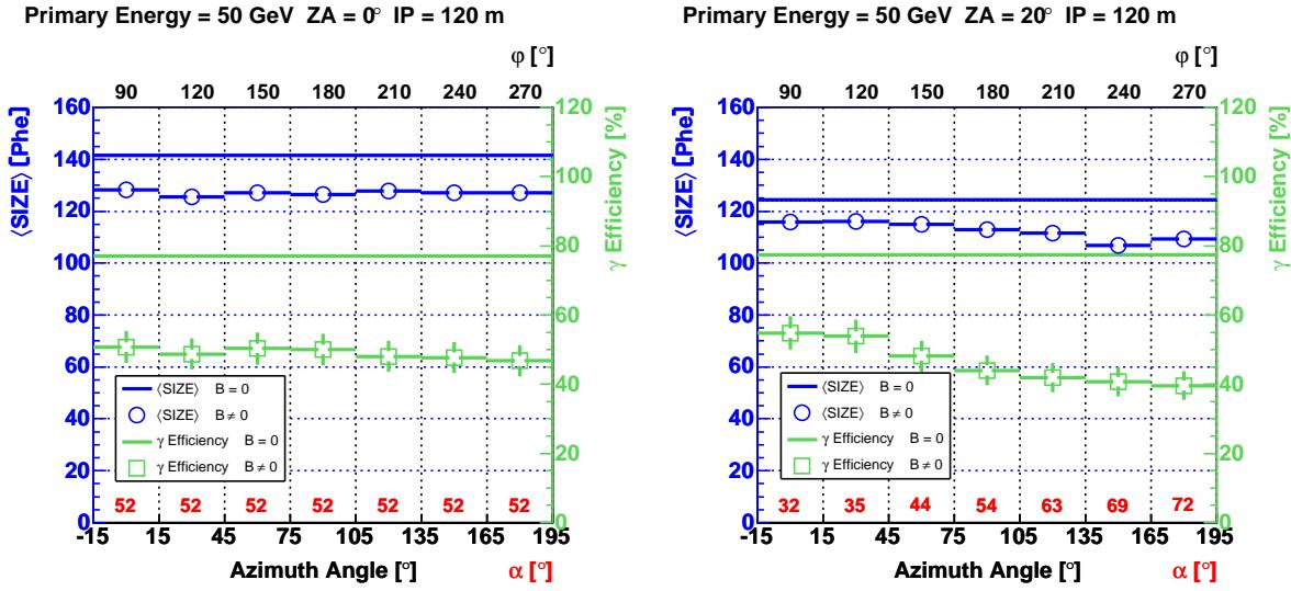
**Figure 201:** The mean value of the image parameter SIZE and the  $\gamma$  efficiency as a function of the azimuth angle for 50 GeV  $\gamma$ -rays and ZA between  $0^\circ$  and  $20^\circ$ . The telescope is always placed at angles  $\varphi = \text{azimuth angle} + 90^\circ$ . The impact parameter was set to  $r = 120$  m. The soft image cleaning was applied.
