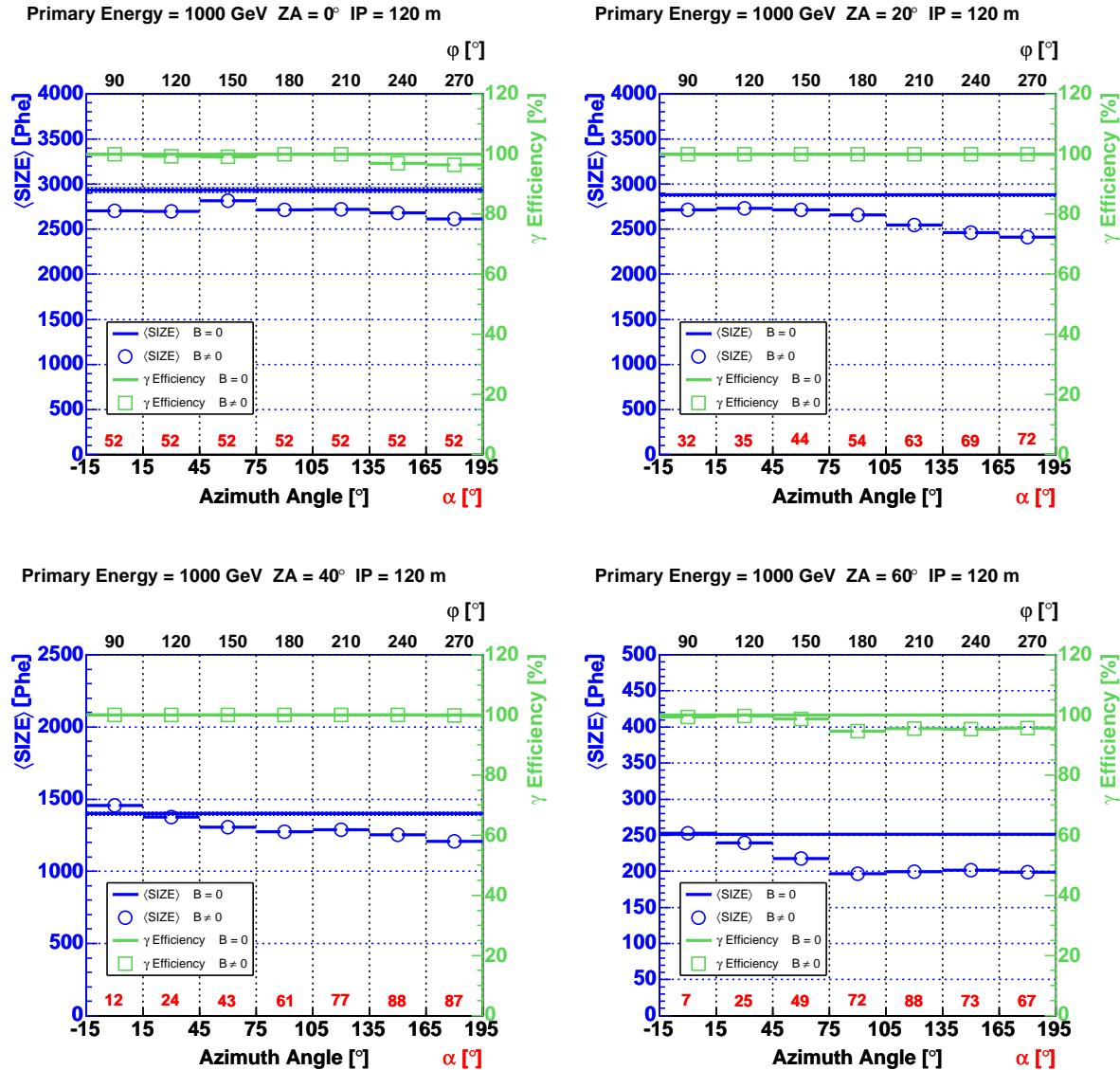
**Figure 213:** The mean value of the image parameter SIZE and the  $\gamma$  efficiency as a function of the azimuth angle for 1 TeV  $\gamma$ -rays and ZA between  $0^\circ$  and  $60^\circ$ . The telescope is always placed at angles  $\varphi = \text{azimuth angle} + 90^\circ$ . The impact parameter was set to  $r = 120$  m. The hard image cleaning was applied.
