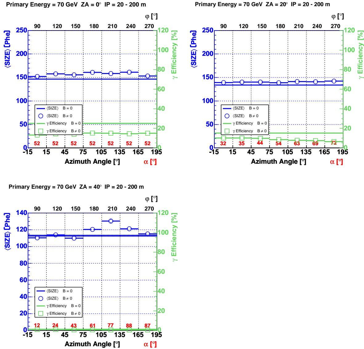
**Figure 204:** The mean value of the image parameter SIZE and the  $\gamma$  efficiency as a function of the azimuth angle for 70 GeV  $\gamma$ -rays and ZA between 0° and 40°. The telescope is always placed at angles  $\varphi$  = azimuth angle + 90°. The impact parameters were set to  $r = 20 \dots 200$  m. The hard image cleaning was applied.
