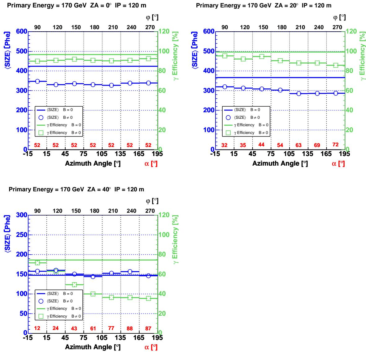
**Figure 207:** The mean value of the image parameter SIZE and the  $\gamma$  efficiency as a function of the azimuth angle for 170 GeV  $\gamma$ -rays and ZA between  $0^\circ$  and  $40^\circ$ . The telescope is always placed at angles  $\varphi = \text{azimuth angle} + 90^\circ$ . The impact parameter was set to  $r = 120$  m. The hard image cleaning was applied.
