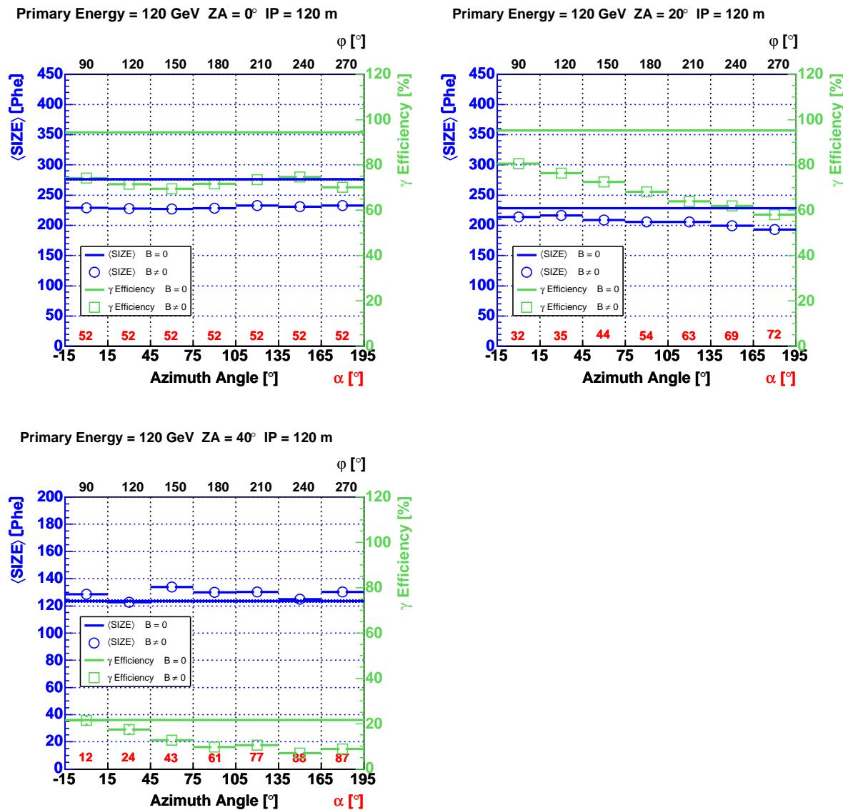
**Figure 205:** The mean value of the image parameter SIZE and the  $\gamma$  efficiency as a function of the azimuth angle for 120 GeV  $\gamma$ -rays and ZA between  $0^\circ$  and  $40^\circ$ . The telescope is always placed at angles  $\varphi = \text{azimuth angle} + 90^\circ$ . The impact parameter was set to  $r = 120$  m. The hard image cleaning was applied.
