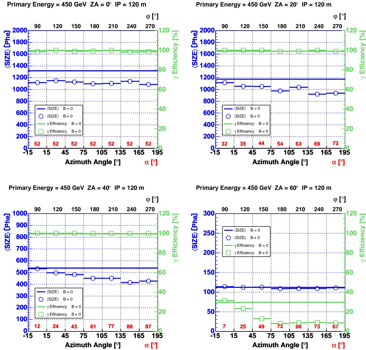
**Figure 211:** The mean value of the image parameter SIZE and the  $\gamma$  efficiency as a function of the azimuth angle for 450 GeV  $\gamma$ -rays and ZA between  $0^\circ$  and  $60^\circ$ . The telescope is always placed at angles  $\varphi = \text{azimuth angle} + 90^\circ$ . The impact parameter was set to  $r = 120$  m. The hard image cleaning was applied.
