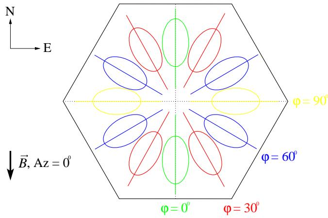
**Figure 81:** The relation between the telescope positions and image orientation in the camera. The green images correspond to the case where the connecting line between shower axis and telescope optical axis is parallel to the north-south direction, i.e. the telescope is situated on the  $x$ -axis of the CORSIKA coordinate system ( $\varphi = 0^\circ$ ). The yellow images are obtained when the telescope is situated on the  $y$ -axis of the CORSIKA coordinate system ( $\varphi = 90^\circ$ ).
