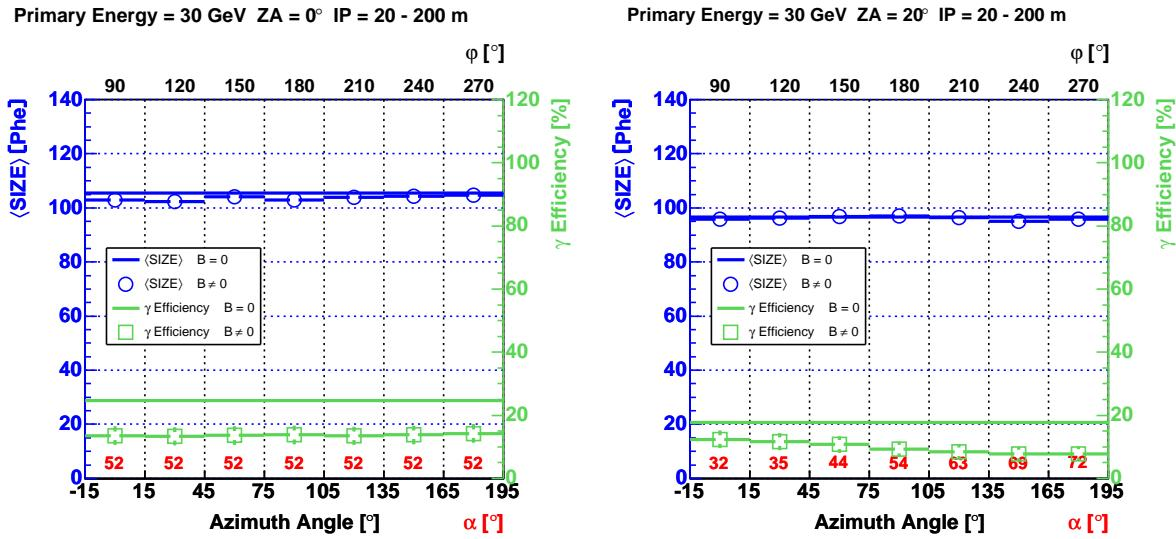
**Figure 200:** The mean value of the image parameter SIZE and the  $\gamma$  efficiency as a function of the azimuth angle for 30 GeV  $\gamma$ -rays and ZA between  $0^\circ$  and  $20^\circ$ . The telescope is always placed at angles  $\varphi = \text{azimuth angle} + 90^\circ$ . The impact parameters were set to  $r = 20 \dots 200$  m. The soft image cleaning was applied.
