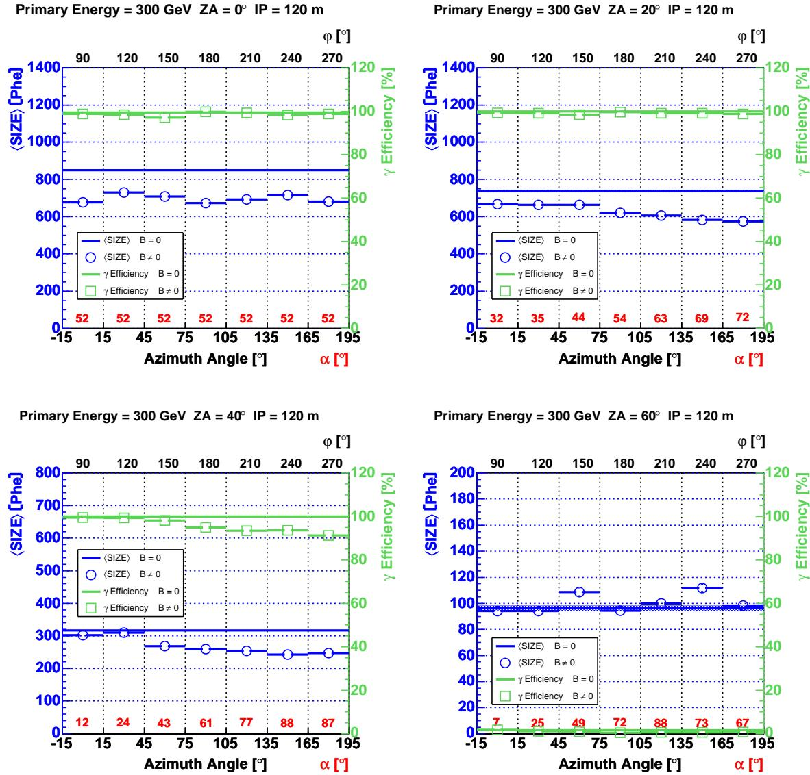
**Figure 209:** The mean value of the image parameter SIZE and the  $\gamma$  efficiency as a function of the azimuth angle for 300 GeV  $\gamma$ -rays and ZA between  $0^\circ$  and  $60^\circ$ . The telescope is always placed at angles  $\varphi = \text{azimuth angle} + 90^\circ$ . The impact parameter was set to  $r = 120$  m. The hard image cleaning was applied.
