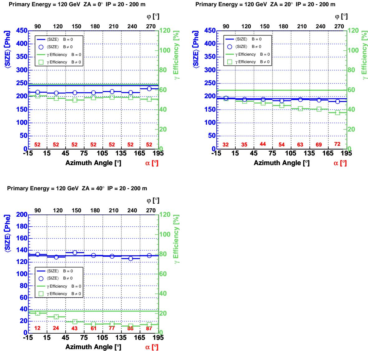
**Figure 206:** The mean value of the image parameter SIZE and the  $\gamma$  efficiency as a function of the azimuth angle for 120 GeV  $\gamma$ -rays and ZA between  $0^\circ$  and  $40^\circ$ . The telescope is always placed at angles  $\varphi = \text{azimuth angle} + 90^\circ$ . The impact parameters were set to  $r = 20 \dots 200$  m. The hard image cleaning was applied.
