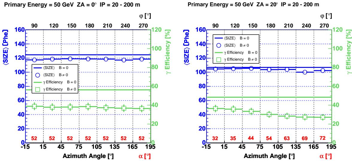
**Figure 202:** The mean value of the image parameter SIZE and the  $\gamma$  efficiency as a function of the azimuth angle for 50 GeV  $\gamma$ -rays and ZA between  $0^\circ$  and  $20^\circ$ . The telescope is always placed at angles  $\varphi = \text{azimuth angle} + 90^\circ$ . The impact parameters were set to  $r = 20 \dots 200$  m. The soft image cleaning was applied.
