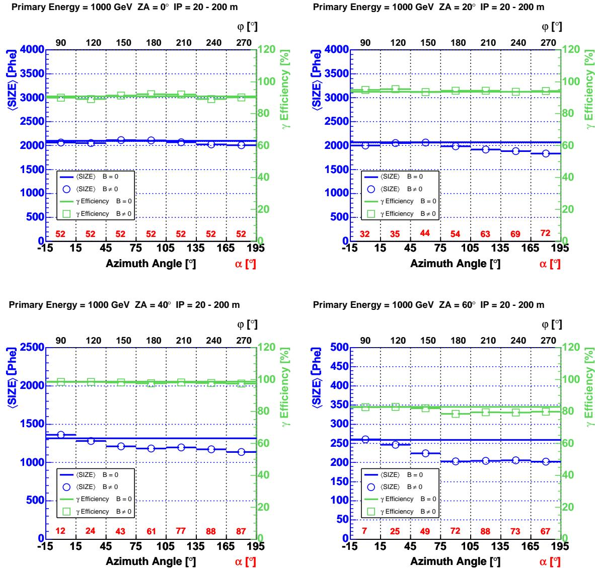
**Figure 214:** The mean value of the image parameter SIZE and the  $\gamma$  efficiency as a function of the azimuth angle for 1 TeV  $\gamma$ -rays and ZA between 0° and 60°. The telescope is always placed at angles  $\varphi$  = azimuth angle + 90°. The impact parameters were set to  $r = 20 \dots 200$  m. The hard image cleaning was applied.
