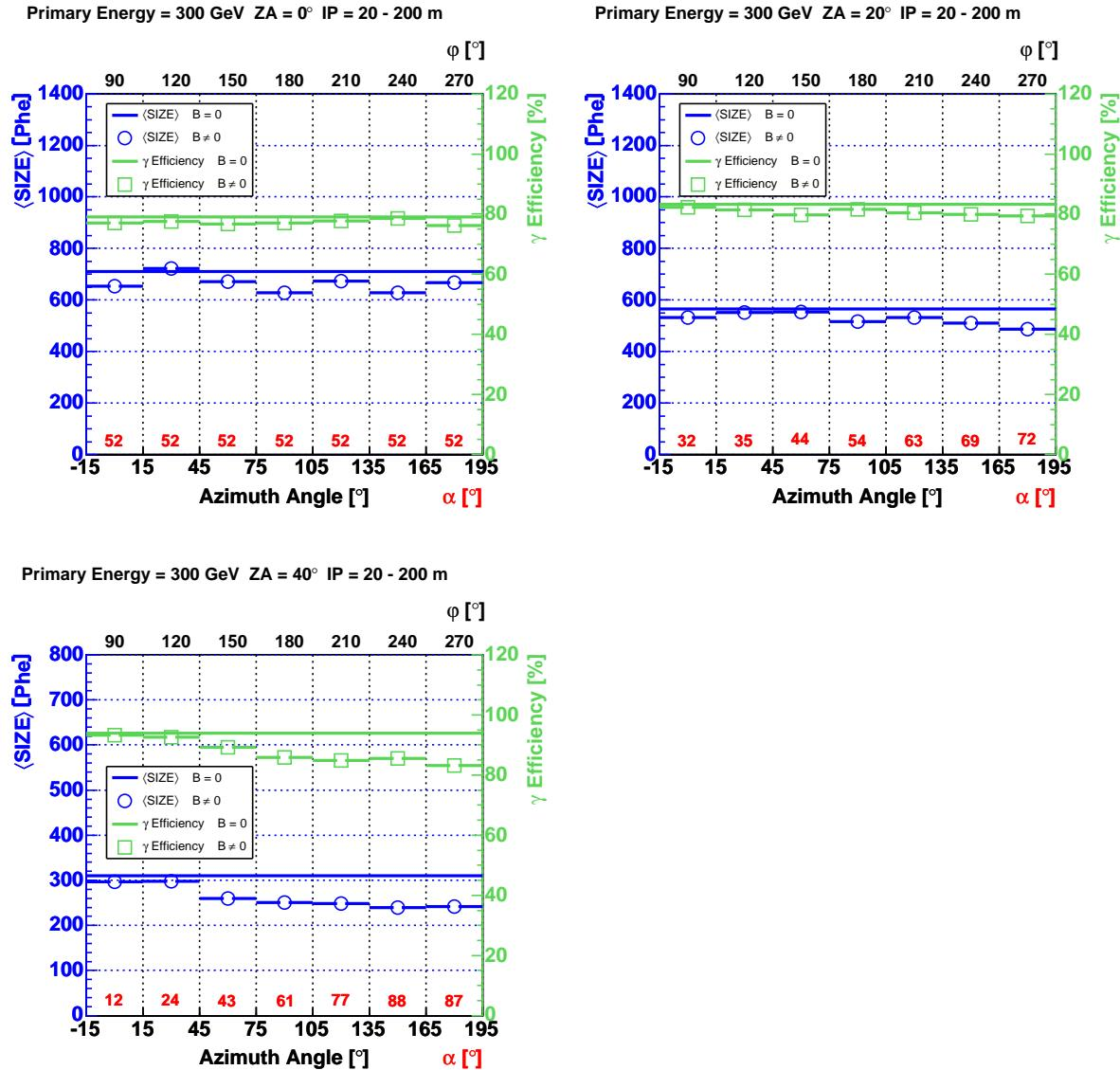
**Figure 210:** The mean value of the image parameter SIZE and the  $\gamma$  efficiency as a function of the azimuth angle for 300 GeV  $\gamma$ -rays and ZA between  $0^\circ$  and  $60^\circ$ . The telescope is always placed at angles  $\varphi = \text{azimuth angle} + 90^\circ$ . The impact parameters were set to  $r = 20 \dots 200$  m. The hard image cleaning was applied.
