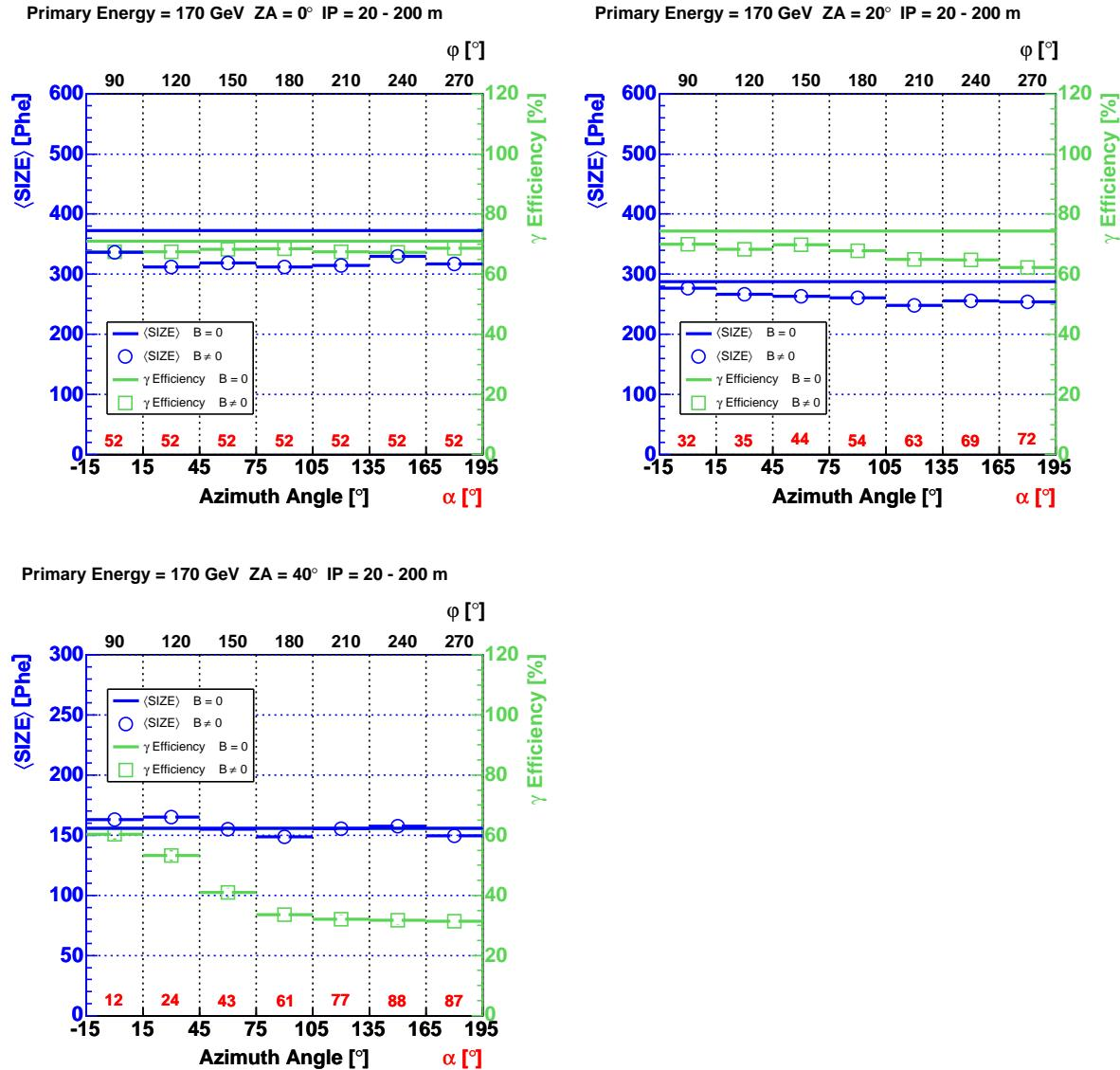
**Figure 208:** The mean value of the image parameter SIZE and the  $\gamma$  efficiency as a function of the azimuth angle for 170 GeV  $\gamma$ -rays and ZA between  $0^\circ$  and  $40^\circ$ . The telescope is always placed at angles  $\varphi = \text{azimuth angle} + 90^\circ$ . The impact parameters were set to  $r = 20 \dots 200$  m. The hard image cleaning was applied.
