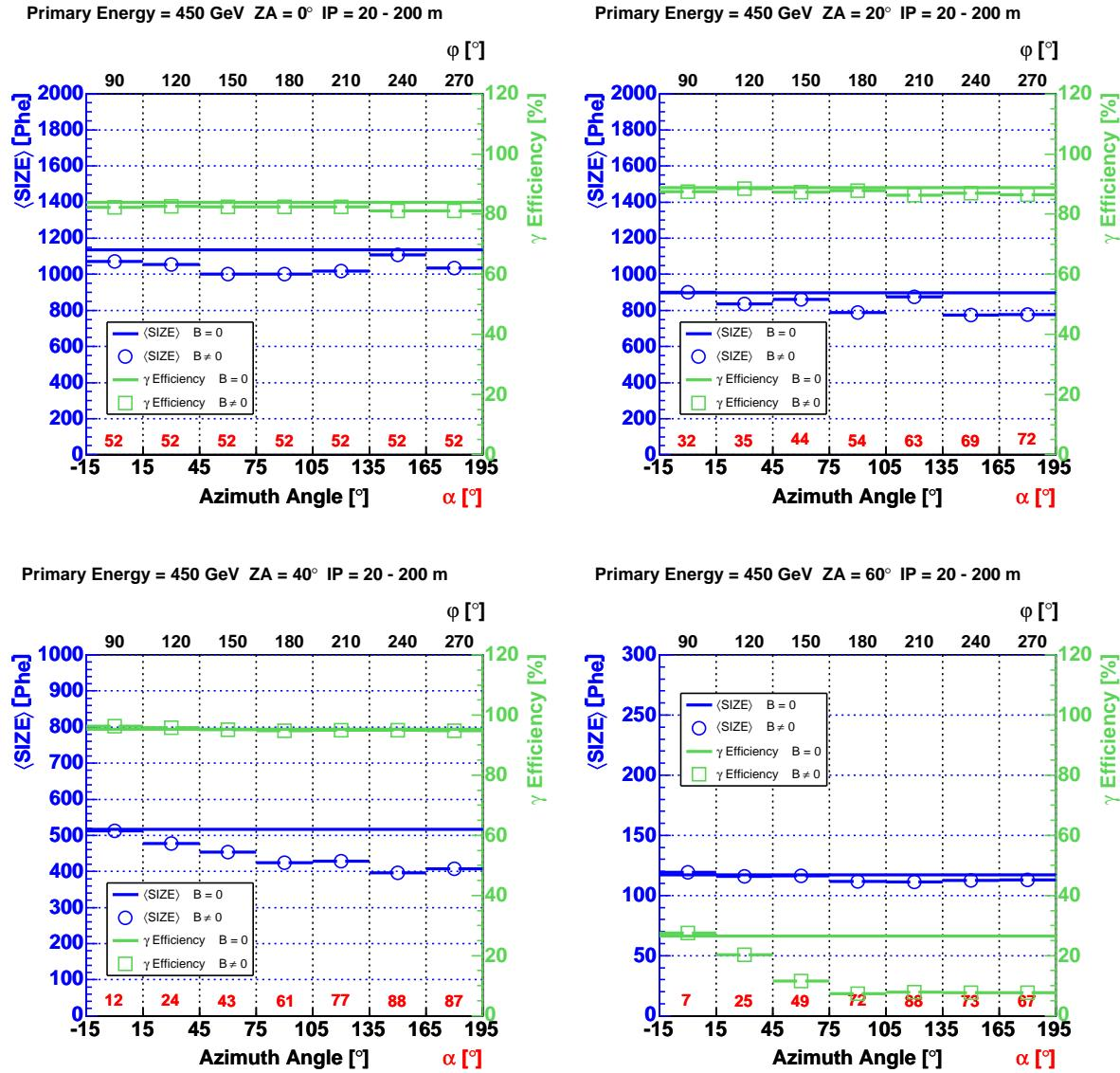
**Figure 212:** The mean value of the image parameter SIZE and the  $\gamma$  efficiency as a function of the azimuth angle for 450 GeV  $\gamma$ -rays and ZA between  $0^\circ$  and  $60^\circ$ . The telescope is always placed at angles  $\varphi = \text{azimuth angle} + 90^\circ$ . The impact parameters were set to  $r = 20 \dots 200 \text{ m}$ . The hard image cleaning was applied.
