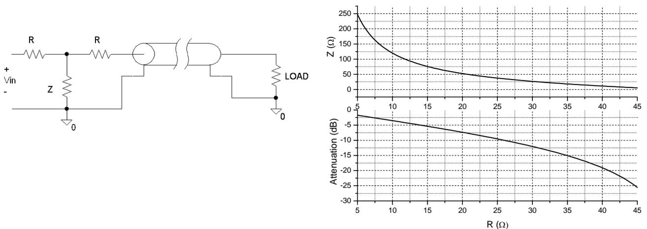
Figure 4. (a) Passive attenuator and transmission line schematic. (b) Graphs used for the design of the desired attenuator (50 Ω matched).
