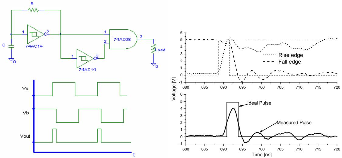
Figure 3. (a) Pulse generator based on the logical glitches (ideal response). (b) Actual generated pulse.
