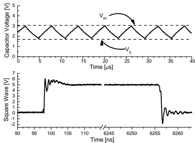
Figure 2: (a) Charge and discharge of the capacitor at the input of the inverter. (b) Rise and fall edges of the square wave.
