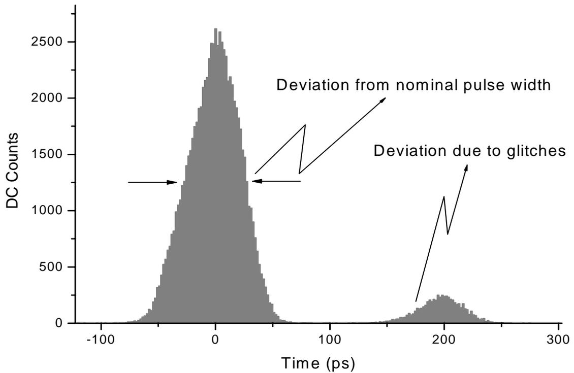
Figure 9. Jitter measurements. The standard deviation from the nominal pulse width is only 39 ps.
