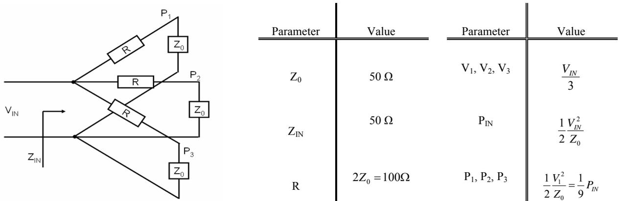
Figure 5. Values of the parameters for a 4 port,  $50 \Omega$  matched, passive power divider.
