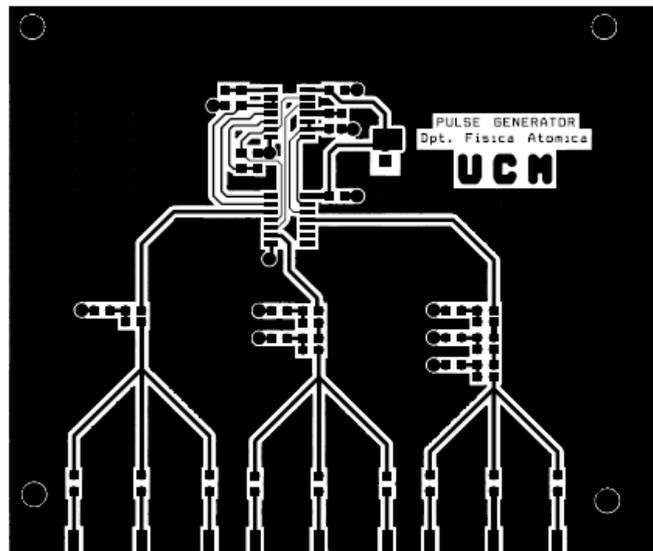
Figure 6. Pulse Generator (a) schematic and (b) layout.
