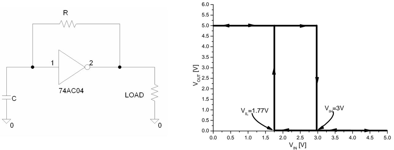
Figure 1. (a) Square wave generator. (b) Hysteresis curve of the 74AC14 HEX inverter.
