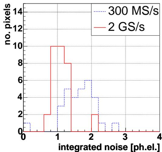
Figure 26: Distributions of the integrated noise in the signal reconstruction window after calibration into photo electrons for the current 300 MSamples/s FADC read-out and using the MUX-FADC read-out.
