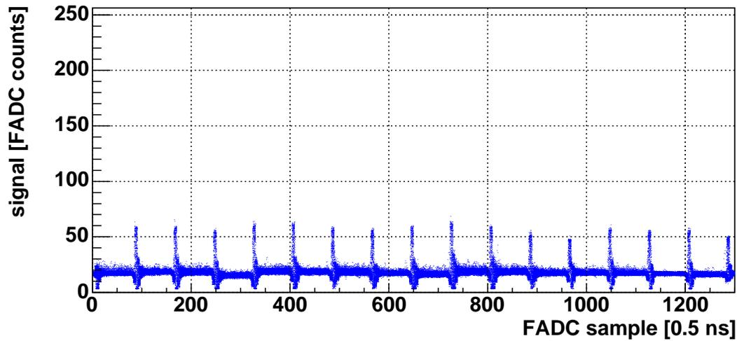
Figure 19: Pedestals: Raw data (1300 samples for 16 consecutive channels) for 120 randomly triggered events overlaid.
