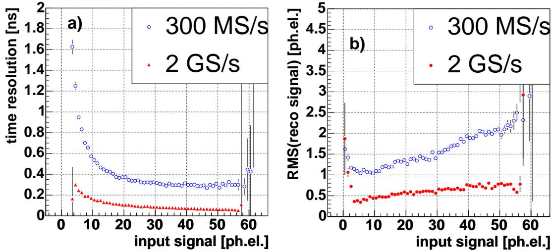
Figure 30: a) Comparison of the pulse arrival time resolution as a function of the input signal size between the current MAGIC 300 MSamples/s FADCs and the 2 GSamples/s FADCs. The time resolution improves by more than a factor of 3 with the new system. b) Comparison of the signal resolution as a function of the input signal with the current 300 MSamples/s MAGIC FADCs and the 2 GSamples/s FADCs system. The signal resolution improves by a factor of about two.
