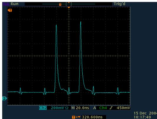
Figure 15: Oscilloscope photo of two consecutive multiplexed signals and the baseline of two empty signal gates.
