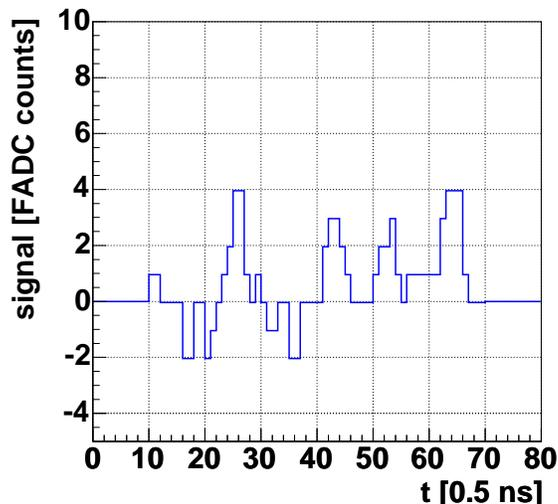
Figure 27: Time structure in a typical pedestal event. The bumps on the baseline might be due to single photo electrons from the light of the night sky.
