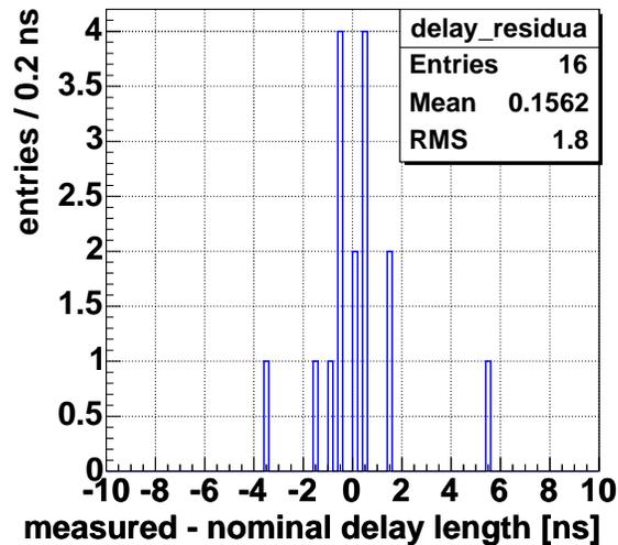
Figure 12: Distribution of the measured deviations of the fiber delay times from the specified channel specific delay of 0...15 ns plus common base delay. – figure to be updated with the results of 600 delays –
