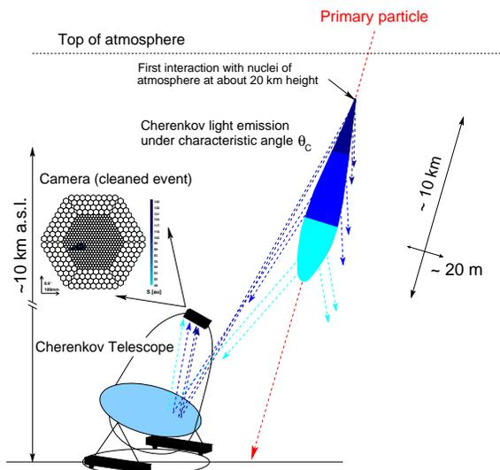
Figure 1: IACT principle: A cosmic high energy gamma ray penetrates the earth's atmosphere and initiates a shower cascade of electrons and positrons, which radiate Cherenkov light. This light is collected and focused onto the camera providing an image of the air shower. Picture taken from [5].
