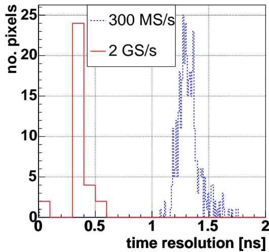
Figure 22: Distributions of the timing resolution for the current 300 MSamples/s FADC read-out and the MUX-FADC read-out. The MUX-FADC system yields an improvement in the timing resolution by more than a factor of three.
