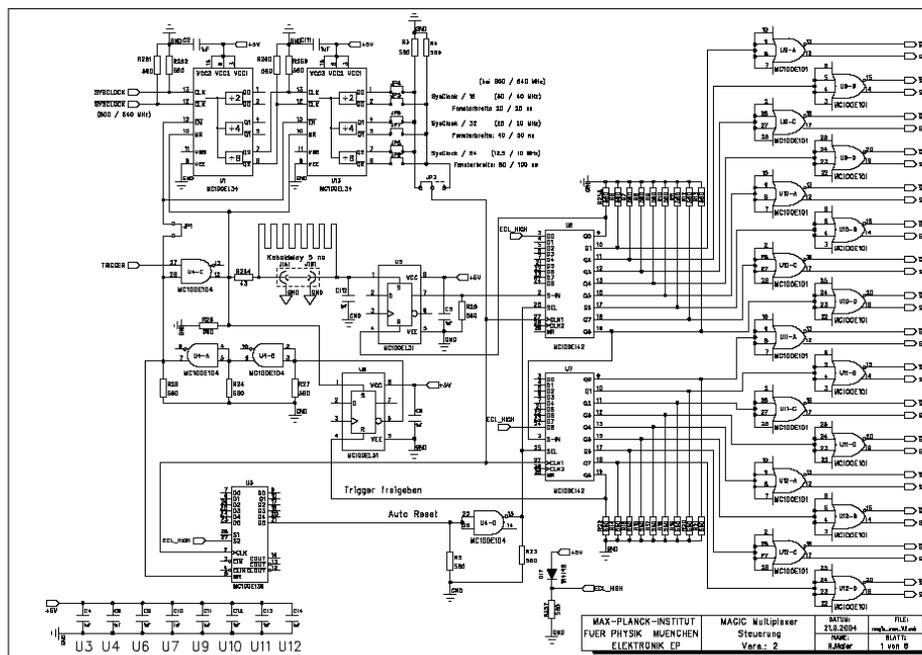
Figure 8: Circuit diagram of the Digital Switch Control circuit (DSC): The trigger initiates a sequence of 16 PECL high levels of 40 ns duration applied consecutively to the switch boards.
