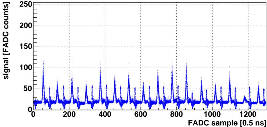
Figure 20: Calibration events: Raw data (1300 samples for 16 consecutive channels) for 120 LED light pulses overlaid.
