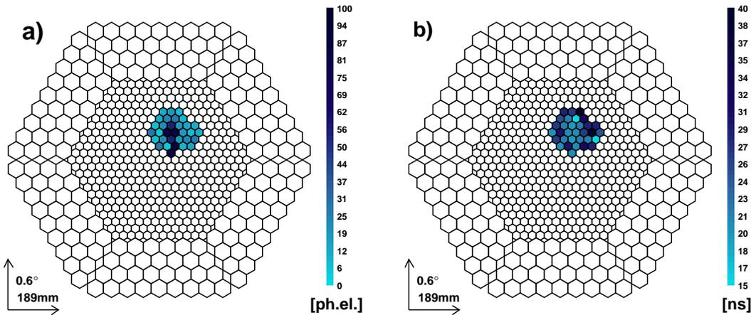
Figure 24: a) Reconstructed signal in photo electrons in the MAGIC PMT camera display and b) calibrated arrival times in ns in the MAGIC camera display for a typical cosmic event.
