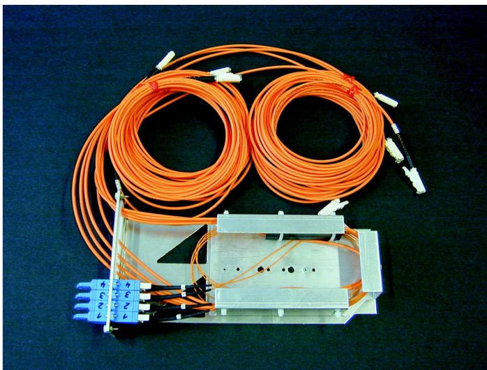
Figure 6: Four channel fiber-optic splitter module, GRIN technology and 50:50 splitting ratio. The outer dimensions are: 235 mm \* 130 mm (3U) \* 35 mm (7HP).
