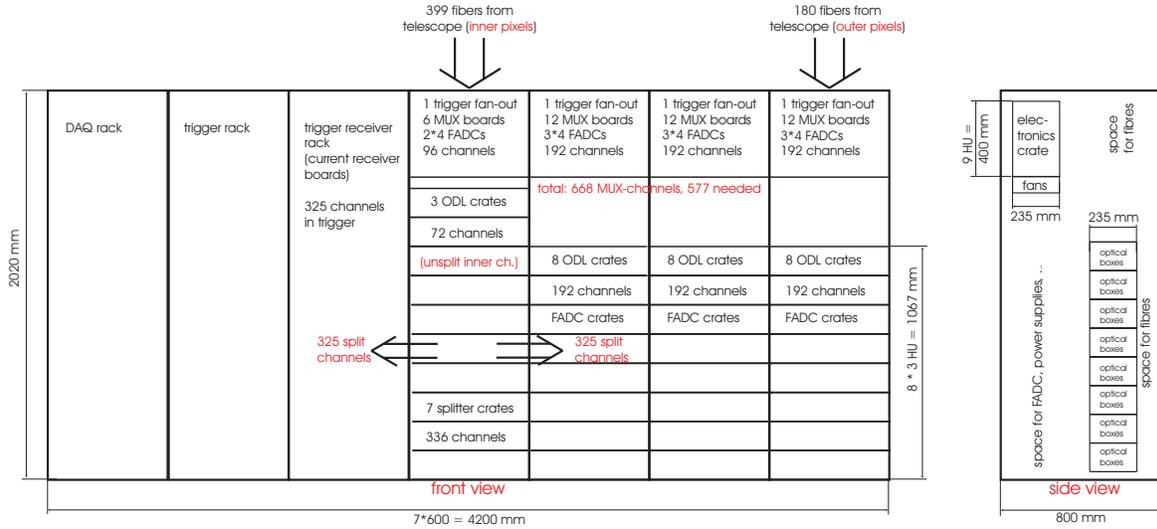
Figure 31: Mechanical Arrangement of the MUX-FADC read-out system.
