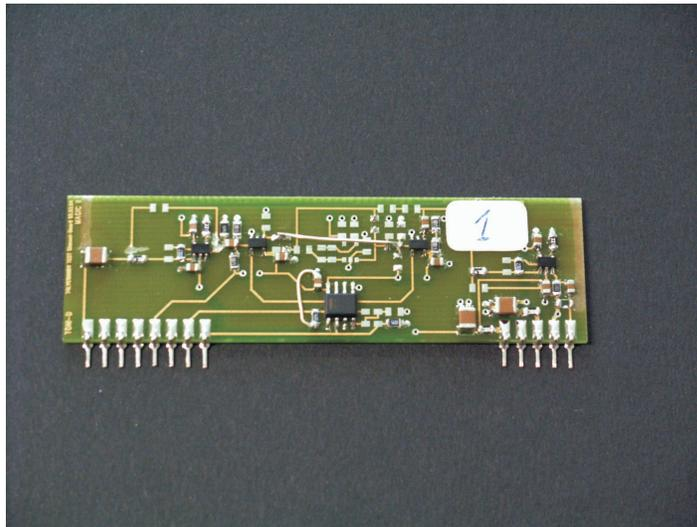
Figure 9: The printed circuit board for fast switching. The switch board contains two ns-MOSFET-switches operated in series. Its mechanical dimensions are 80 mm \* 20 mm \* 5 mm. – picture to be updated, latest production prototype –
