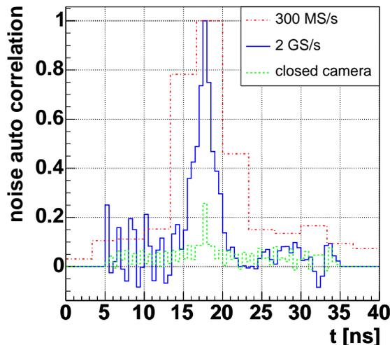
Figure 25: Noise autocorrelation function with respect to a fixed FADC sample for the current MAGIC readout chain with 6 ns pulse shaping, the MUX-FADC read-out with open camera and closed camera, normalized to the pedestal RMS of the opened camera.
