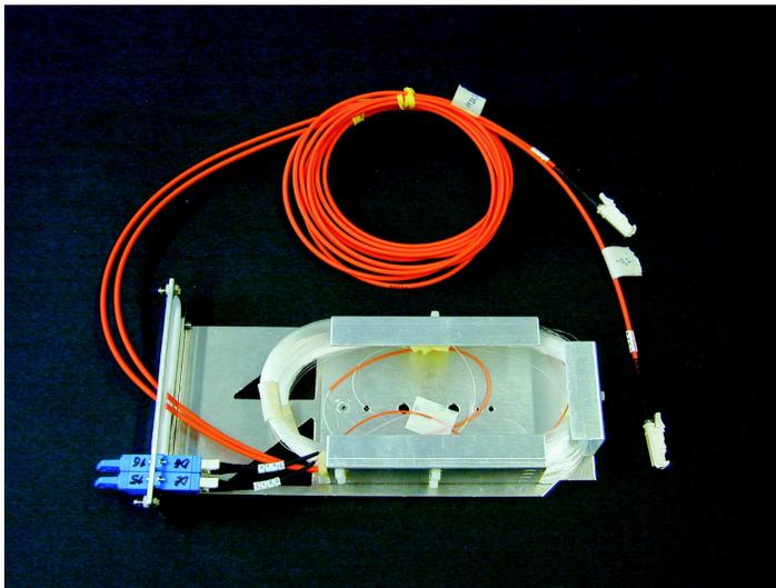
Figure 5: Two channel fiber-optic delay module of 142 and 150 m length, corresponding to a delay of 710 and 750 ns, respectively. Mechanical dimensions: 235 mm \* 130 mm (3U) \* 35 mm (7HP).
