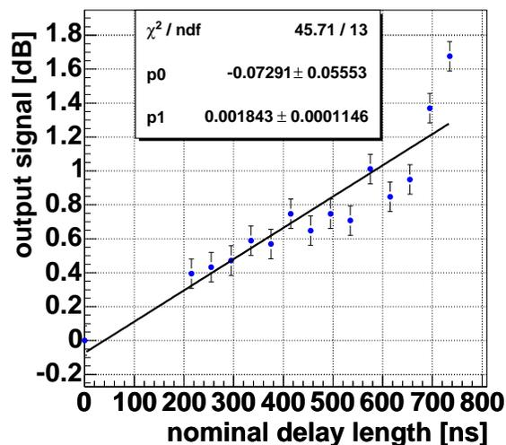
Figure 13: Signal Attenuation in the optical delay lines. The signal attenuation coefficient is determined to be  $(1.8 \pm 0.1)$  dB/ $\mu\text{s}$ .
