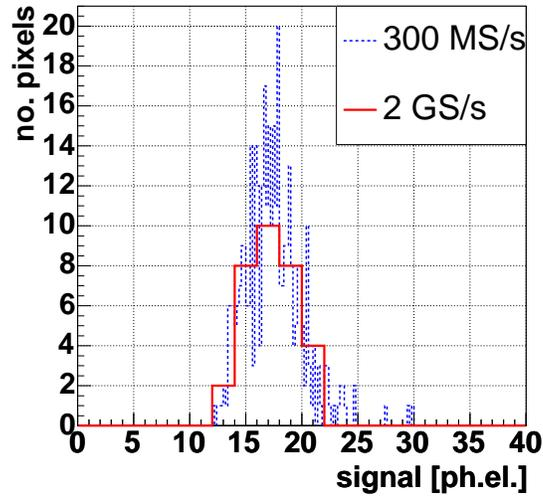
Figure 21: Distributions of the mean reconstructed number of photo electrons in the PMTs of the MAGIC camera from the LED pulser for the current 300 MSamples/s FADCs and the MUX-FADCs. Both read-out systems yield the same average number of photo electrons.
