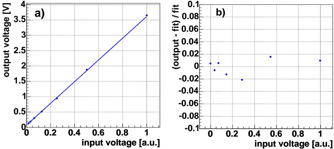
Figure 16: a) Output signal amplitude of the MUX board as a function of the input signal after the PIN diode as measured at the monitor output. b) Residua of the linearity of the MUX board as a function of the input signal after the PIN receiver diode as measured at the monitor output. The deviations are less than 2%. – plots to be updated, last production prototype of the MUX board, 3dB steps, log scale –
