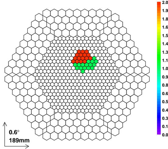
Figure 18: Location of the selected 32 channels in the MAGIC PMT camera.
