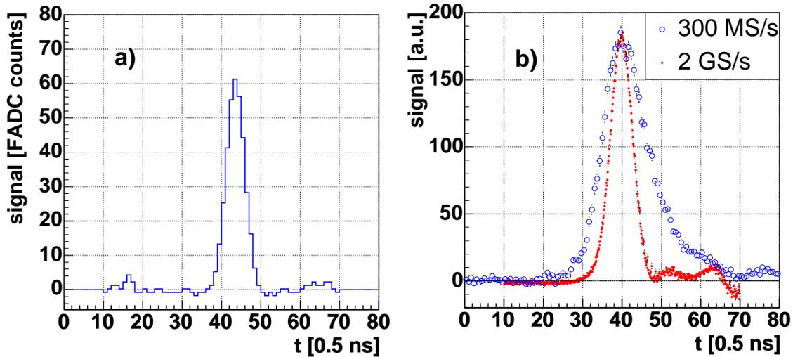
Figure 23: a) Pulse shape in a single pixel for a typical cosmics event after pedestal subtraction. b) Comparison between the mean reconstructed pulse shapes recorded with the current MAGIC FADCs (red triangles) and with the MUX-FADCs (blue circles).
