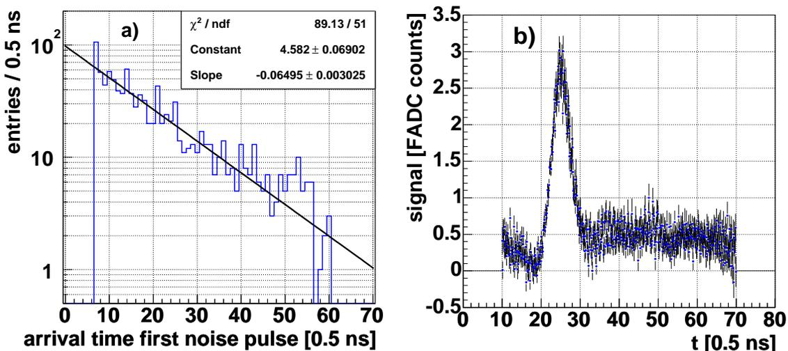
Figure 28: a) Arrival time distribution of the first “bump” on the pedestal baseline. The bumps are arriving randomly in time with a rate of  $(0.13 \pm 0.01)\text{ns}^{-1}$ . b) Average reconstructed shape of the LONS noise “bumps”.
