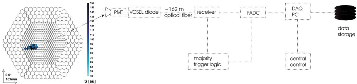
Figure 3: Current MAGIC read-out scheme: the analog PMT signals are transferred via an analog optical link to the counting house where after the trigger decision the signals are digitized by using a 300 MHz FADCs system and written to the hard disk of a DAQ PC.
