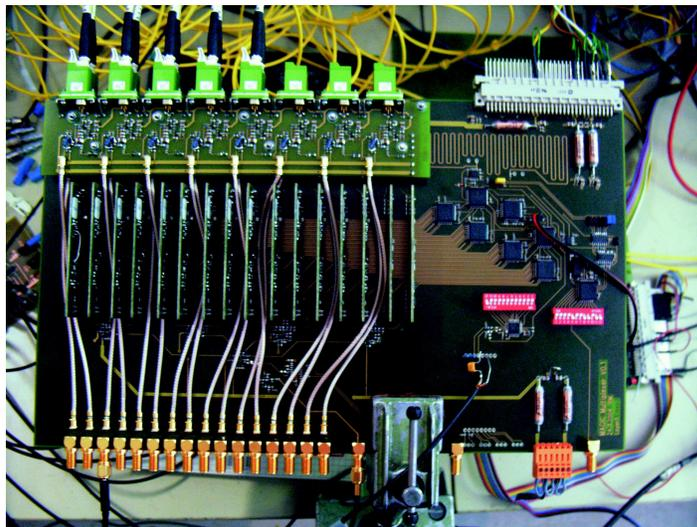
Figure 7: Photo of the printed circuit board for analogue signal multiplexing: It consists of a trigger input, 16 opto-electric converters, 16 monitor signal outputs, the Digital Switch Control circuit (DSC), 16 daughter switch boards and two summing stages. The overall size is 370 mm (9 U) \* 220 mm \* 30 mm (6 HP). – picture to be updated, latest production prototype, black background –
