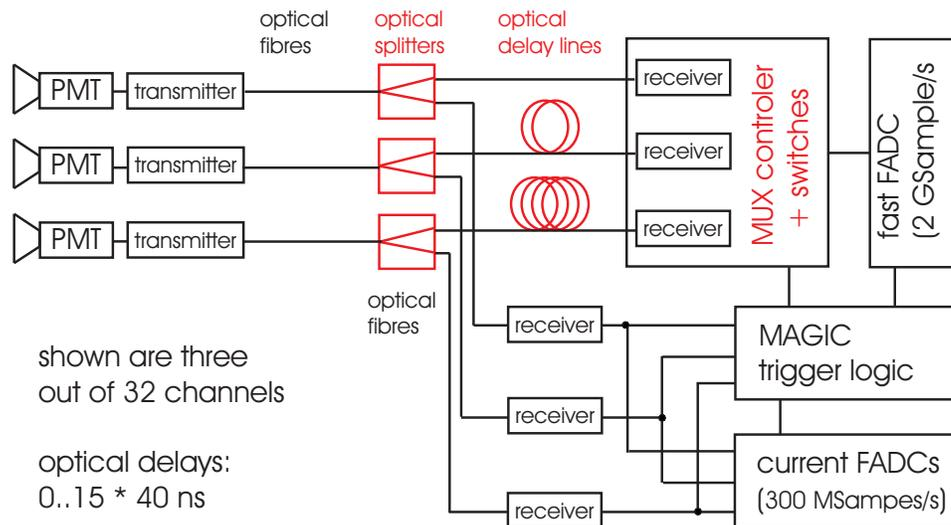
Figure 17: Block diagram of the integration of the MUX-FADC prototype read-out in the current MAGIC FADC read-out. Shower images are simultaneously recorded with the ultra-fast MUX-FADC system and with the current MAGIC FADCs. The MAGIC trigger logic provides a trigger for the MUX electronics as well as for the ultra-fast FADCs.
