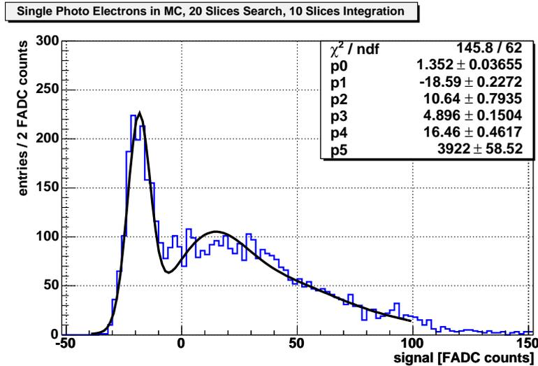
Figure 29: Reconstructed single photo electron spectrum of a simulated pedestal run. The left peak is the pedestal.
