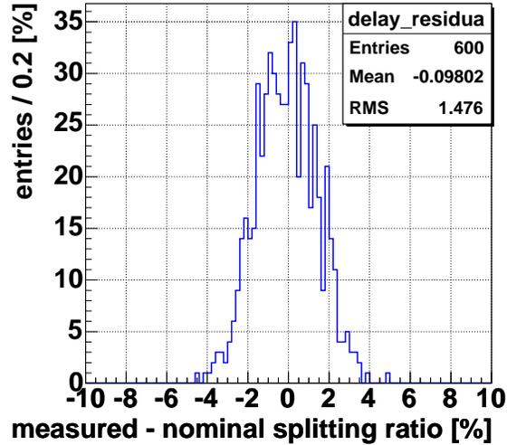
Figure 14: Distribution of the measured deviations of the GRIN-type fiber-optic splitters from the specified 50:50 splitting ratio. – figure to be updated with the results of all 352 GRIN-splitters –
