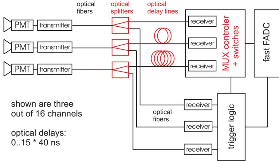
Figure 4: Schematic diagram of the multiplexed fiber-optic ultra fast FADC read-out. Part of the analog signal that arrives via the fiber-optic link from the PMT camera is branched off and fed into a majority trigger logic. The other part of the signals is consecutively delayed in optical fibers. One channel after the other is connected to the ultra fast FADC using fast switches. Thereby the noise from the other channels is efficiently blocked.
