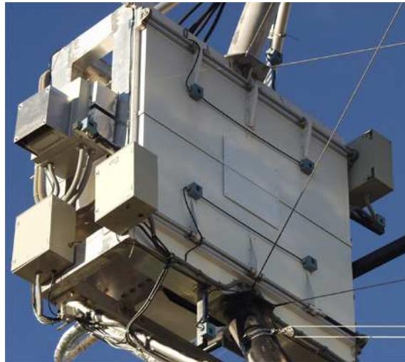
Figure 2.1: The two Al-plates mounted on the camera lids acting as a projection screen for the lasers of the AMC.
