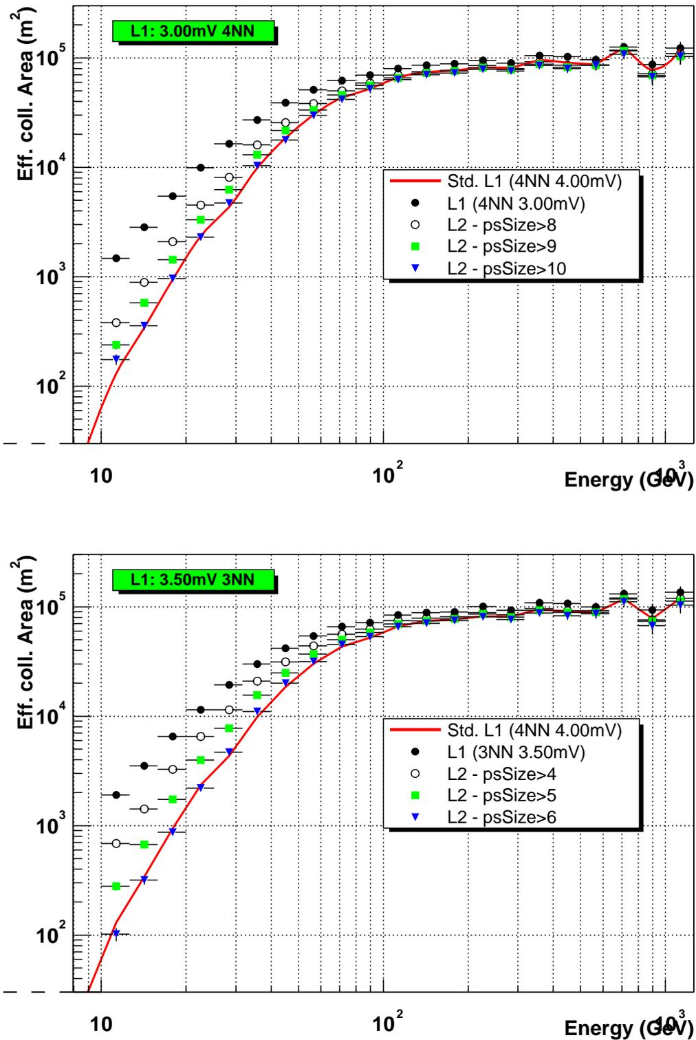
Figure 7: The effective collection area for gamma events, for some L1 trigger topologies and discriminator thresholds (from top to bottom: 3.00mV-4NN, 3.50mV-3NN), and for some pseudo-size cuts. As a reference the collection area of the “standard” trigger condition (L1: 4.0mV-4NN; no L2T cuts) is shown as a solid line.
