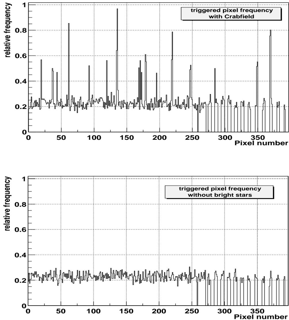
Figure 3: Trigger rate for single pixels in the trigger area with (top) and without (bottom) the bright stars in the Crab Nebula starfield (L1: 3.00mV-4NN; 192 triggered events). 25 hot pixels can be identified; 6 of them are isolated while the others are grouped in clusters of 2-4 pixels. The present plot is affected by a bug in the reflector program which smears the photons in the camera, possibly producing an higher number of hot-pixels [8].
