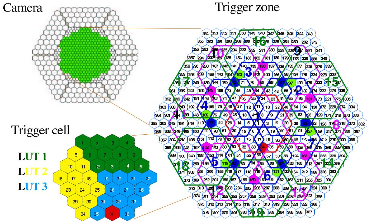
Figure 1: The trigger zone, divided into 19 trigger cells, and a scheme of one cell with its three LUTs.
