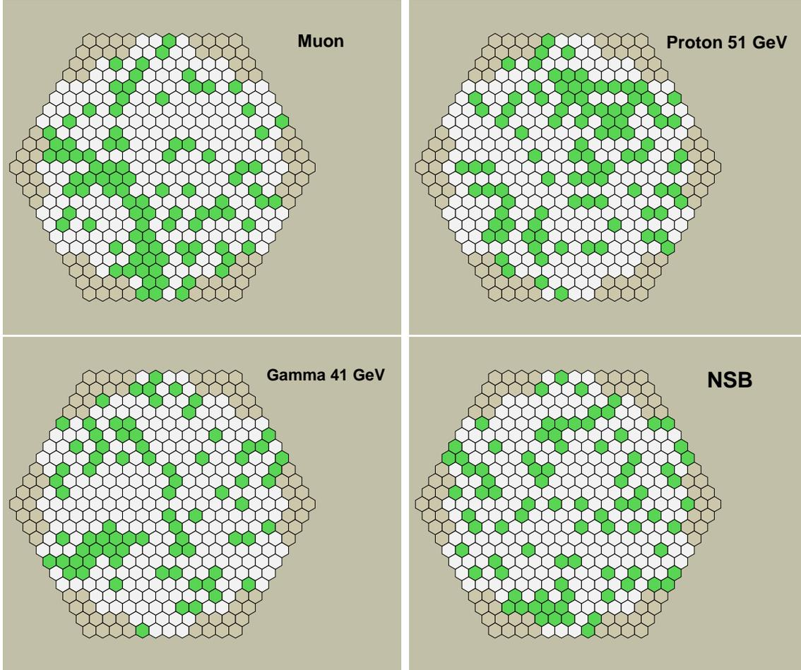
Figure 4: Examples of trigger events produced by a muon (top-left), proton (51 GeV, top-right), gamma (41 GeV, bottom-left) and pure NSB (bottom-right). A night sky background signal produced by 3.00 mV-4NN L1 trigger conditions is added in all events.
