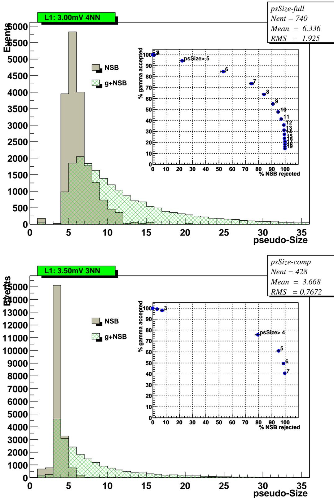
Figure 5: The pseudo-Size distribution, for gamma (green, dashed) and pure NSB (grey, solid) events, for some L1 trigger topologies and discriminator thresholds (from top to bottom: 3.00mV-4NN, 3.50mV-4NN). The inset shows the gamma-acceptance vs. NSB-rejection for different pseudo-size cuts. The value of the cut is reported next to each point.
