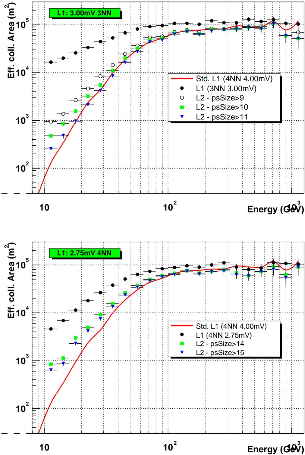
Figure 8: The effective collection area for gamma events, for some L1 trigger topologies and discriminator thresholds (from top to bottom: 3.00mV-3NN, 2.75mV-4NN), and for some pseudo-size cuts. As a reference the collection area of the “standard” trigger condition (L1: 4NN; Disc. thr.: 4.0mV; no L2T cuts) is shown as a solid line.
