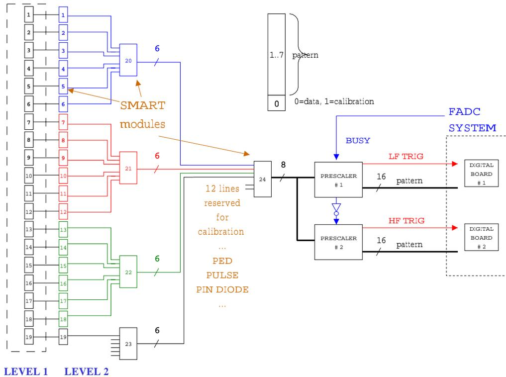
Figure 2: The L2T architecture. The trigger pattern (8 bits) is fed into the prescaler module that generates the trigger signal for the FADC system which starts the acquisition.
