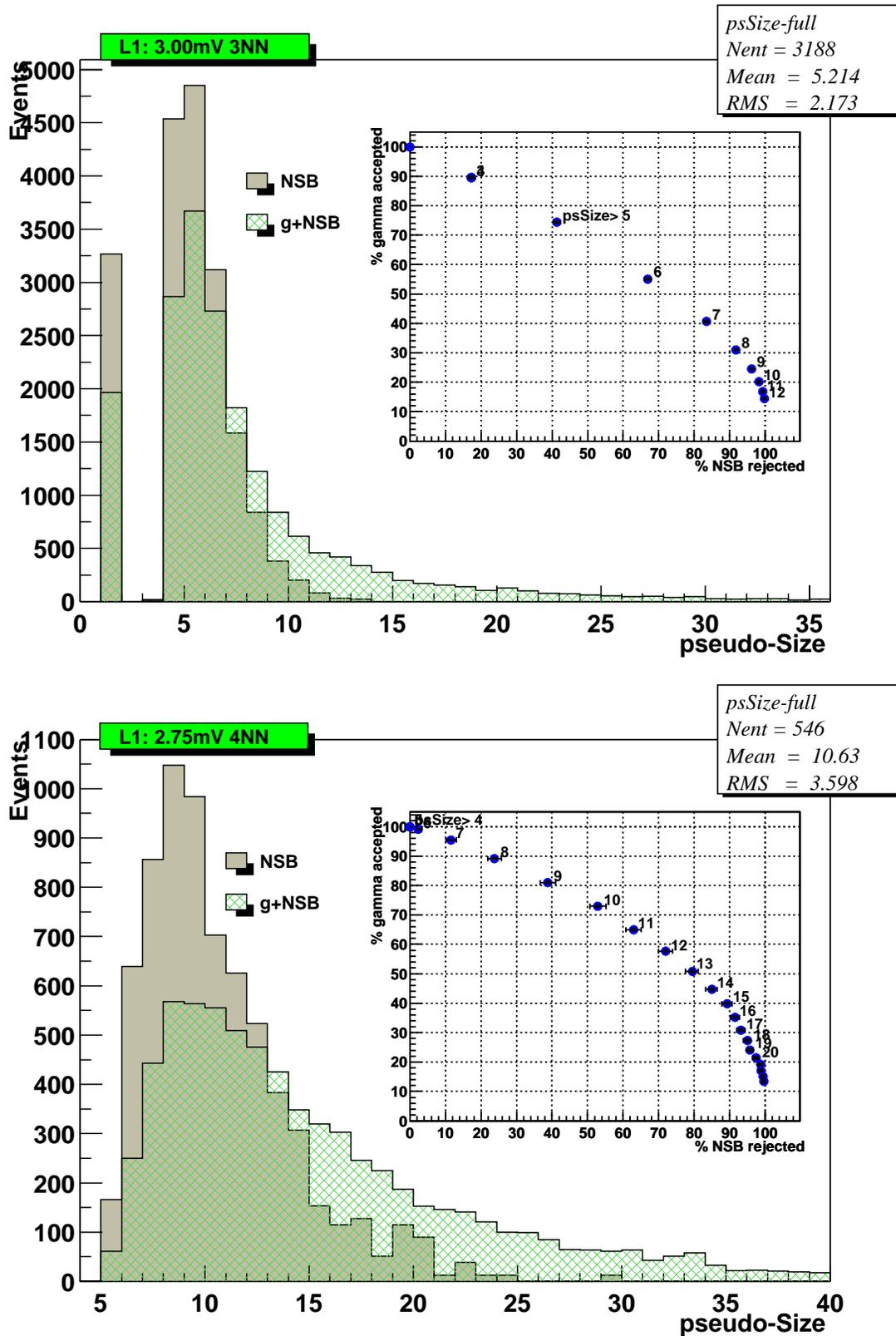
Figure 6: The pseudo-size distribution, for gamma (green, dashed) and pure NSB (grey, solid) events, for some L1 trigger topologies and discriminator thresholds (from top to bottom: 3.00mV-3NN, 2.75mV-4NN). The inset shows the gamma-acceptance vs. NSB rejection for different pseudo-size cuts. The value of the cut is reported next to each point.
