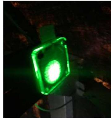
**Figure B.4:** Attached target to the telescope frame illuminated by the expanded laser beam.
