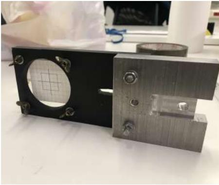
**Figure B.3:** Attachable target for laser alignment during the day.
