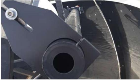
(a) Bent down laser guidance tube
