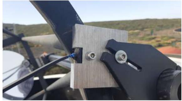
(b) Bent aluminium cross of the detector mount
