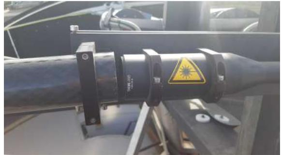
(d) Misaligned transition from laser beam expander to guidance tube
