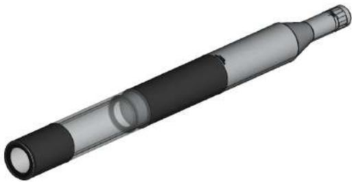
**Figure B.1:** CAD image of the new guidance tube with inserted baffle rings to reduce stray light.
