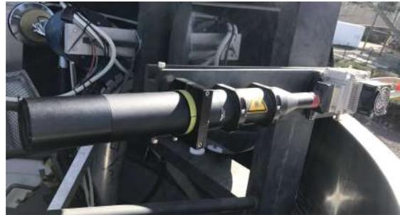
**Figure B.2:** Implemented tube setup directly mounted at the laser plate and screwed on to the beam expander with no gap.
