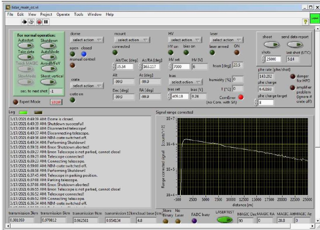
Figure 3.3: Screenshot of the LabVIEW user interface to control the LIDAR.
