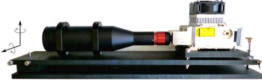
**Figure 3.17.:** Photograph of the transmitter unit of the LIDAR system. It consist of a 532 nm laser and a 20× beam expander mounted onto a custom made bench revolvable around two axis for the light beam adjustment.
