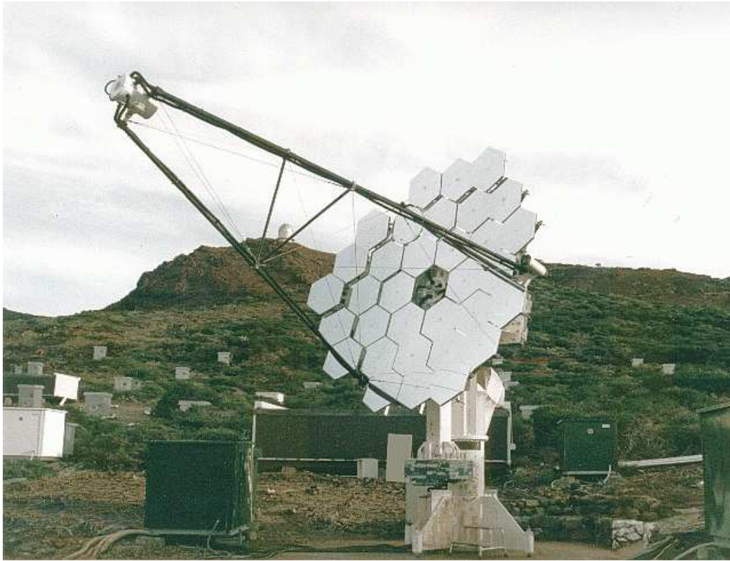
Figure 4.17: Photograph of the HEGRA prototype telescope CT1 after the installation of the new all-aluminium hexagonal mirror elements.
