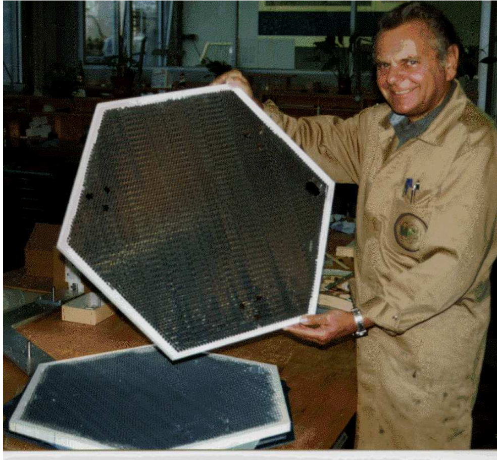
Figure 4.16: Photograph of production of a HEXCELL spacer for a hexagonal mirror element.
