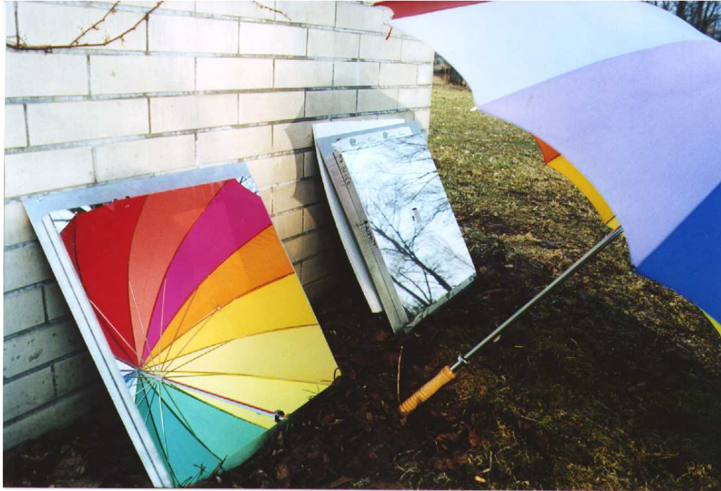
Figure 4.19: Photograph illustrating the quality of two preproduction mirror elements.
